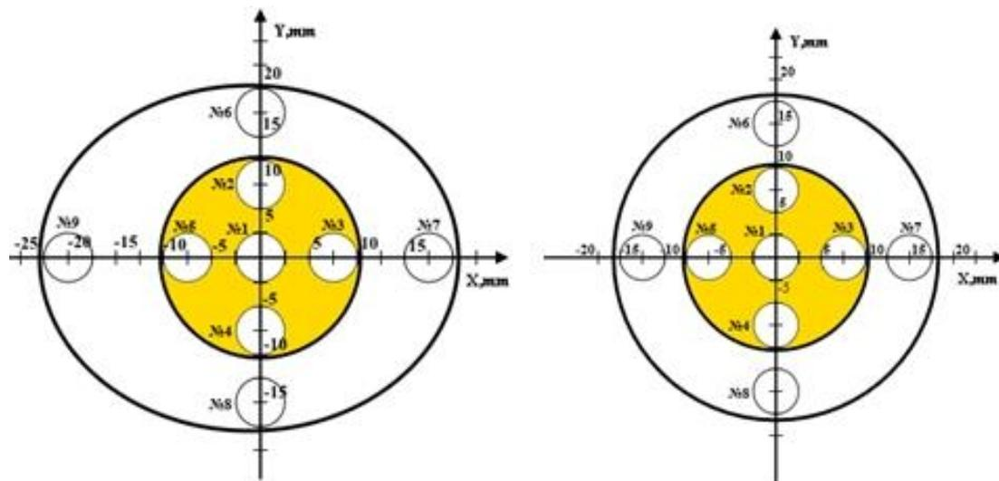
Fig 4: Location of TLD dosimeters (5 mm in diameter) at vertical (right) and the horizontal section of the hens' eggs.
