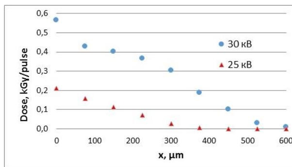
**Fig 2: Distribution of the electron beam AD in the depth in the polyethylene at a different charging voltage on the accelerator URT-0.5.**
