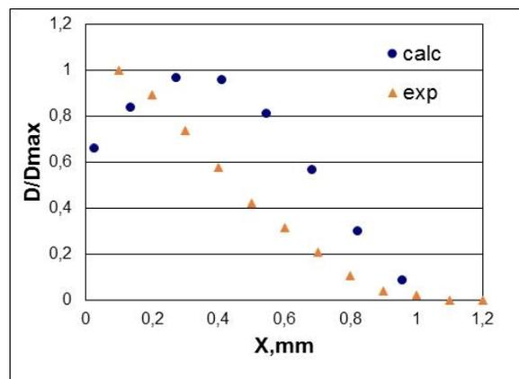
**Fig 1: Measured experimentally and calculated distribution of absorbed dose (AD) in the depth in the polyethylene.**
