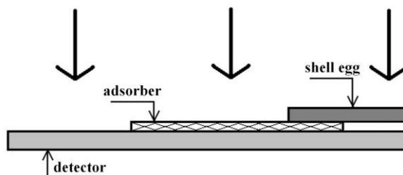
**Fig 3: The geometry of the irradiation under the electron beam dosimetry.**
